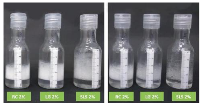
Figure 1: Comparing foam formation properties exhibited by a 2% solution of Ramnocare (RC), a 2% solution of lauryl glucoside (LG) and a 2% solution of sodium lauryl sulfate (SLS). Ramnocare exhibited the same foam formation effect as the lauryl glucoside solution. The SLS solution produced higher foam volume, but the foam was less dense.
