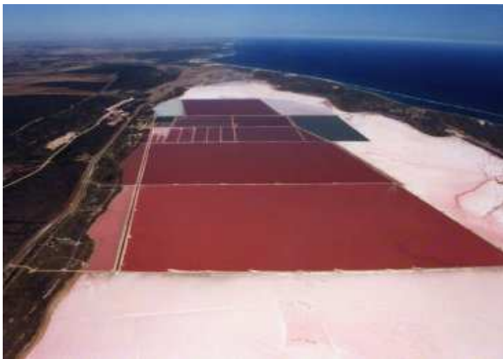
The large open ponds used for the culture of Dunaliella salina at Hutt Lagoon, Western Australia, by Cognis Nutrition and Health. The largest ponds are about 250 ha in area.
